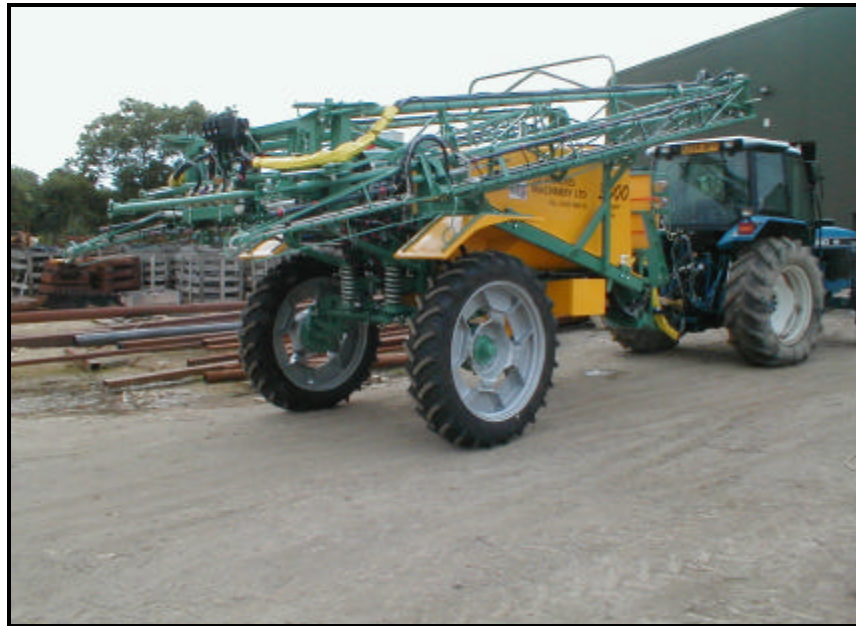
ASA 4000 litre 24m Suspended Trailed Sprayer
