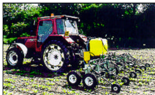
Miser Airtec Band Sprayer 6, 12, or 18 row or bed system, 350 litre tank covers 14 Ha per fill
