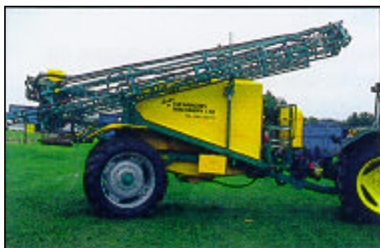
ASA Heavy Duty Trailer Sprayer with steering axle 3000 - 4000 Litre capacity Boom widths 18 - 36 Metres Airtec or Conventional
